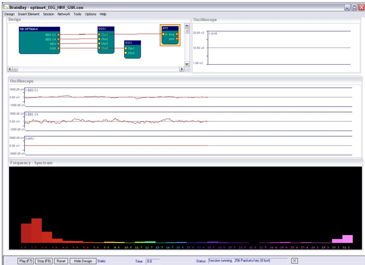
This configuration features two EEG channels with 125 Hz sampling rate, one ECG/HRV channel and one GSR channel. A FFT spectrum analysis of channel 1 is displayed, and the raw signals of both EEG channels and the ECG channel are shown in an Oscilloscope. The GSR values are shown in a separate Oscilloscope with slower trace.
